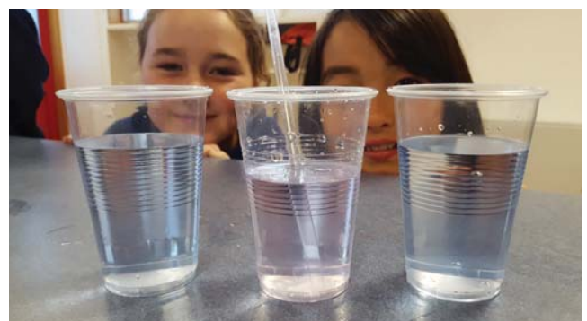
Diluted red cabbage indicator. Control cups on the left and right, the test cup with carbon rich breath blown into it through a straw in the centre.
